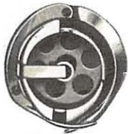
Figure G Correct Position of Hook for Re- moving Gib Screws and Gib.
