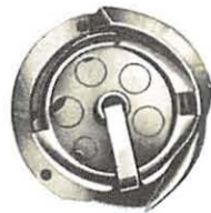
Figure I Relative Position of the Latch to the Point of the Hook For Removing Bobbin Case.
