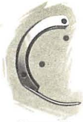
Figure H Gib and Screws Removed for Bobbin Case Replacement.
